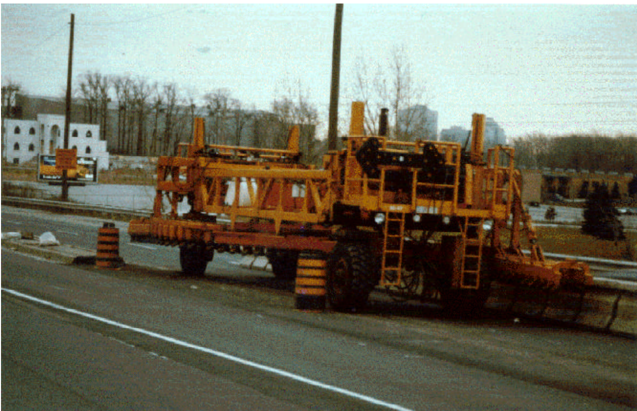
"Quickchange TTV" parked at layby area near end of movable barrier system. The barrier was relocated twice daily during a major construction stage when deck width was restricted to three lanes total.
