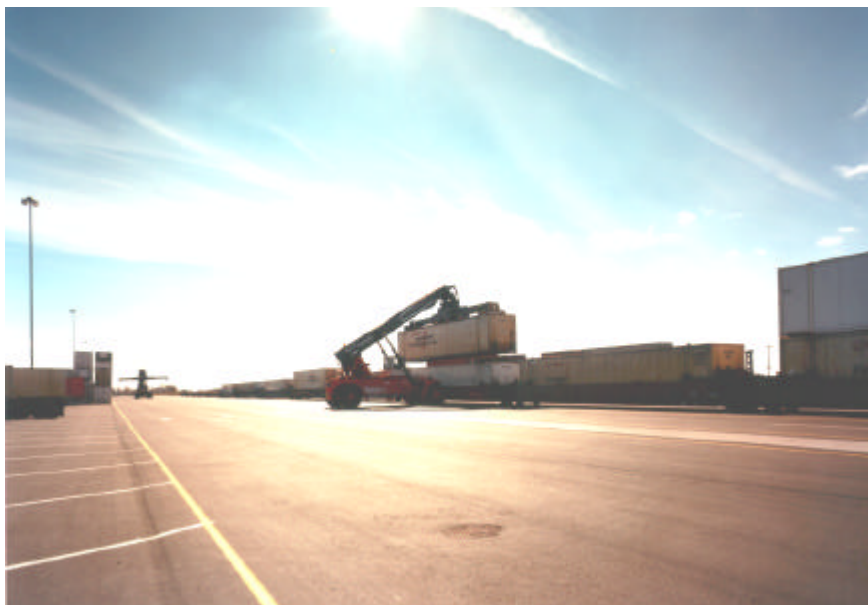
Toplifter operation used to place containers.
